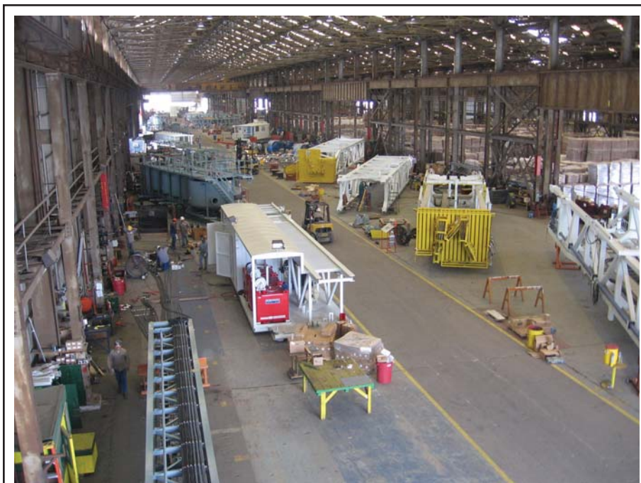
A six-point “road map” was developed to achieve the goals of minimizing the number of steps in each part of the rig manufacturing process at Helmerich & Payne’s assembly facility, and reducing the variation in each step. As a result, the assembly facility experienced dramatic reductions in safety incidents, cycle time and labor cost.
